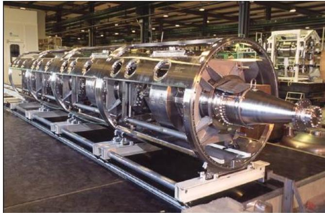
Figure 4: Four cavities make up one cryomodule. In total there are four cryomodules in the LHC, two per beam.
