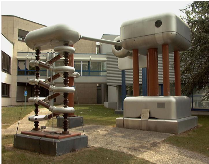
Figure 1: Cockcroft-Walton generator (600 kV) built by Philips, used in 1964 as a high-voltage supply for the 3 MeV Linac pre-injector to the proton synchrotron. Image by CERN.
