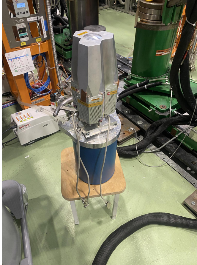
Figure 3.6: Dismounted Miniball HPGe detector crystal with the cooling system visible, showing the compact cryostat design and electrical feedthroughs.
