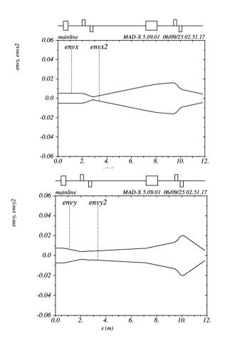
beam shape – very similar and 1.8 cm in the x direction and 2.0 cm in the ydirection.
