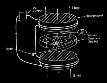
modern cyclotrons – a sequence of magnets and cavities – Azimuthally Varying Focusing(AVF) cyclotrons, relativistic energies, magnetic field increases with the radius
