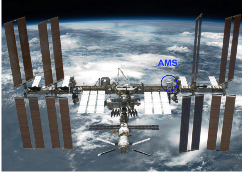
Figure 3.1: AMS mounted on the ISS, tilted 12^\circ from zenith to avoid the rotating solar arrays, and designed to operate for the Station's lifetime [26].
